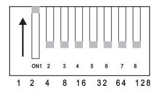
Dip switch dip downward is open meaning, as the drawing showing the dmx-512 address is setting "1"
